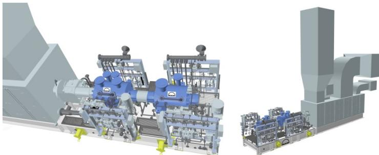
*MAN compressor train with two RB35 barrel-type compressors, driven by a 13MW gas turbine from Solar Turbines*
